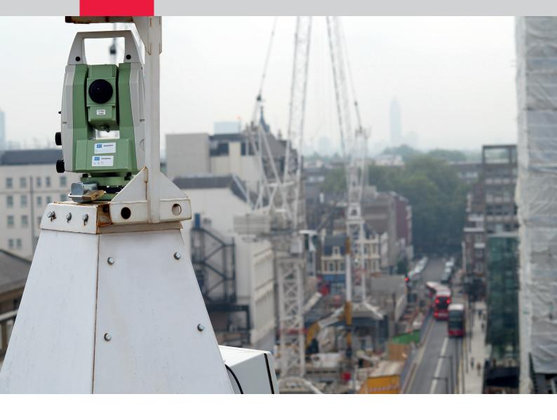
solutions play an important role in securing the success of this new railway line by monitoring structures and the degree of earth settlement.
