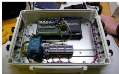
Datalogger configuration for Inclination Sensors and Anemomete
