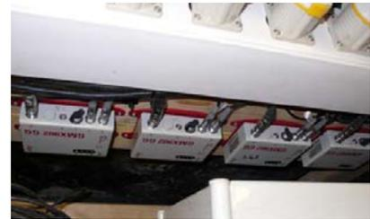
4 x GMX902GG GNSS Receivers inside the slip form rig.
