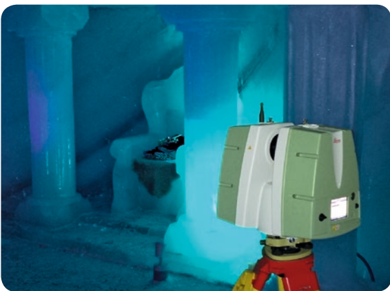
■ The ScanStation P20 scanning the Ice Palace.
