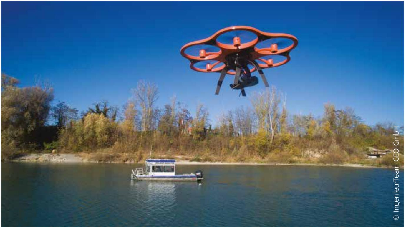
Focusing on surveying engineering technologies, IngenieurTeam GEO was contracted to determine the remaining volume in Knobel-Bau's quarries. By creating georeferenced orthophotos and digital terrain models using the Aibotix Aibot X6 unmanned aerial vehicle (UAV), the firm was able to present the current situation in detail and provide an effective inventory reduction plan.
