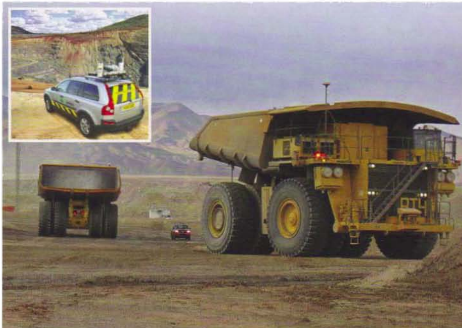
From the large to the small: High-precision GPS technology plays a role in both these Komatsu 930E-4 haul trucks, configured for autonomous operation at Rio Tinto's Australian iron ore mines; and in MineMapper, a system that combines laser scanning with GPS location that can be mounted on almost any vehicle to generate highly accurate terrain measurements while on the move.
