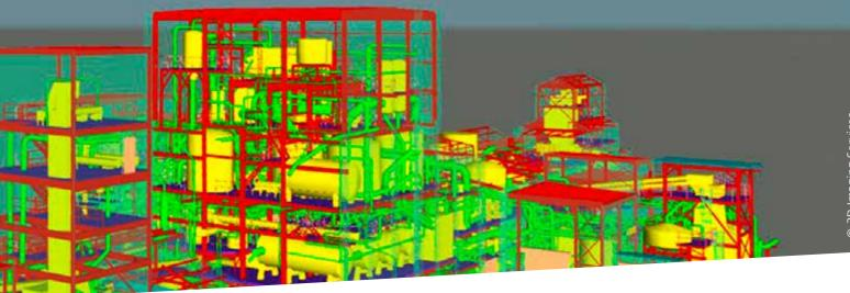
its line of sight at a rate of up to 1 million points per second and producing a point cloud, this laser scanner empowered a crew of two to document the plant in one day. In that time, they were able to capture the data from 65 scan positions. James explains, "One person could have physically accomplished the job, but we used two to ensure safety."
