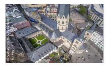
Detailed aerial images were collected using a UAV from areas where the scanners could not be positioned, such as for external roof or tower areas. This resulted in approximately 3,200 facade photos used for corrections and processing. Around 500 distinct points from the scanned point clouds were determined as the foundation points to link the images together.
