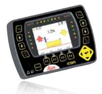
Leica iCON grade 32 2D Grading solution Easy monitoring of the blade position. Main function keys for easy operation.
