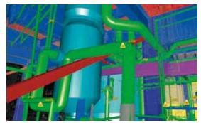
The automated Pipe Run feature lets users select points on connected, straight pipe sections, and the system automatically models a best fit pipe run with elbows in
