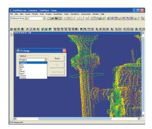
Intelligent point fitting tools assit in finding flange faces at pipe centerlines. This ensures users can identify exact and accurate tie-points, a very important part of modeling as-built piping.
