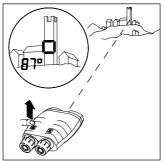
Sight the object with the pointing circle, then release the azimuth key while holding the Laser Locator steady.
