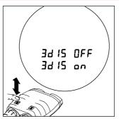
The function "3dIS on" allows up to 3 distances to be displayed from a single measurement (see page 12).
