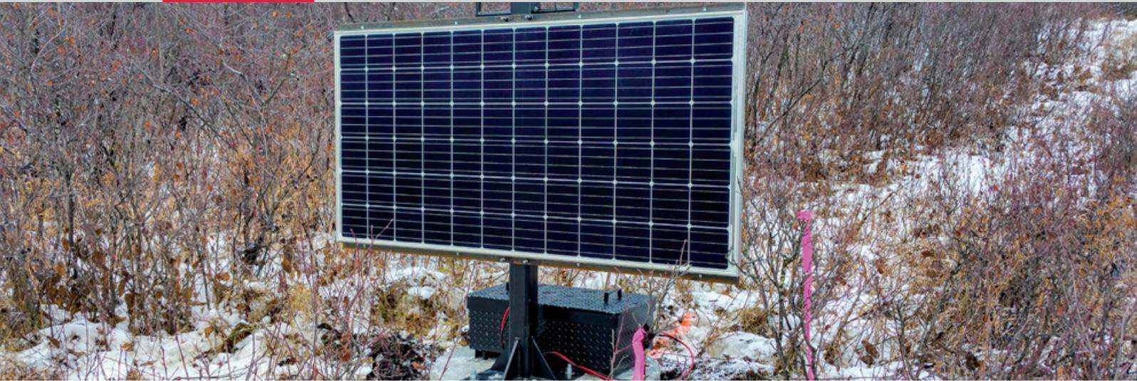
“System uptime is very important to us and is a big differentiator for our monitoring solutions,” says Rutledge. “Our GM30s have internal memory that can be partitioned so that part of it operates on a first-in first-out basis. That means that even if there is a communication failure, or if the ministry’s server goes down, all of the data collected at that site is available from this partition for a year or so. We automatically retrieve it and process it once the system is back online.”
