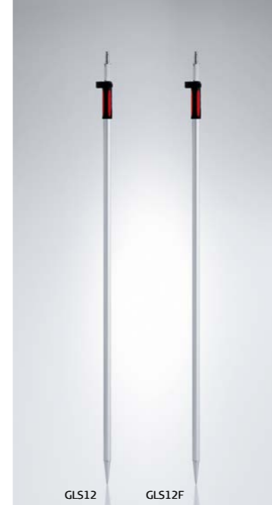
GLS12, Telescopic pole Pole with snap locks to prevent any pole slip. Suitable for the GRZ122 reflector together with GNSS antenna. Graduated in cm, min. length 1.39 m, extendible to 2.0 m, weight 950 grams. Order No: 754391
