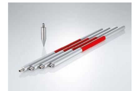
GLS115, Mini pole Set of four screw-together sections and point with 1/4" threads. Suitable for GMP111, GRZ101 and GPR105 reflectors. Provides prism heights of 10, 40, 70, 100 or 130 cm. For prisms without bubble a additional clip on bubble is available (GLI115, 747895). Order No: 642106
