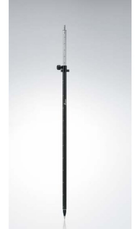
GLS101, Telescopic pole Carbon / aluminium reflector pole with twist lock and pin lock to prevent any pole slip. Graduated in cm and ft. Min. length 1.31m, extendible to 2.3m, weight 1,230 g. Order No: 865472
