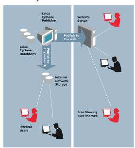
Leica Cyclone Publisher is used to compress point cloud data and create panoramic images with accurate measurable data for viewing and mark-up with the free TruView Internet Explorer plug-in. This data, much like PDF, can be made available on an internal network, over the web or distributed on a CD or DVD. The TruView plug-in makes accessing this data easy for any class of user with no training required.
