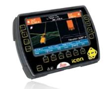
Leica iCON excavate 41 3D Excavating solution Full visual guidance of the bucket see the job as you want. Menu keys give the operator an easy overview of functions.
