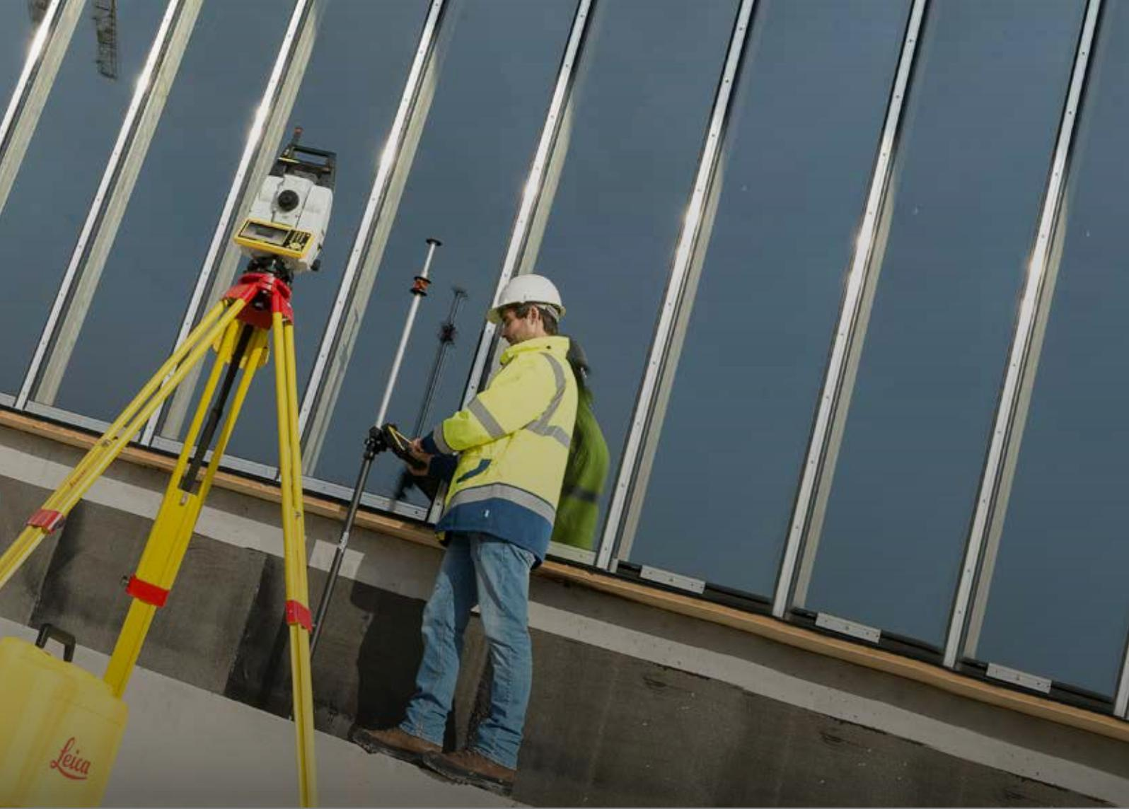
surroundings are no reason to lose our user's target. In case of interruption of lock by co-workers, other trades, or equipment on a congested site, re-lock to the prism occurs automatically and quickly.
