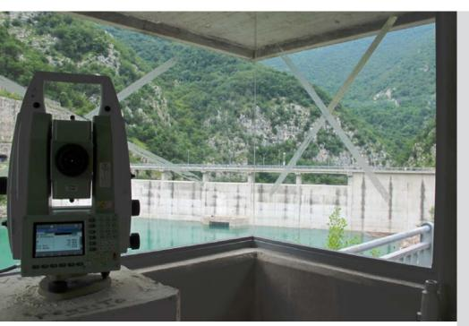
Automatic monitoring system with dual station operation with the Leica TM30 station.
