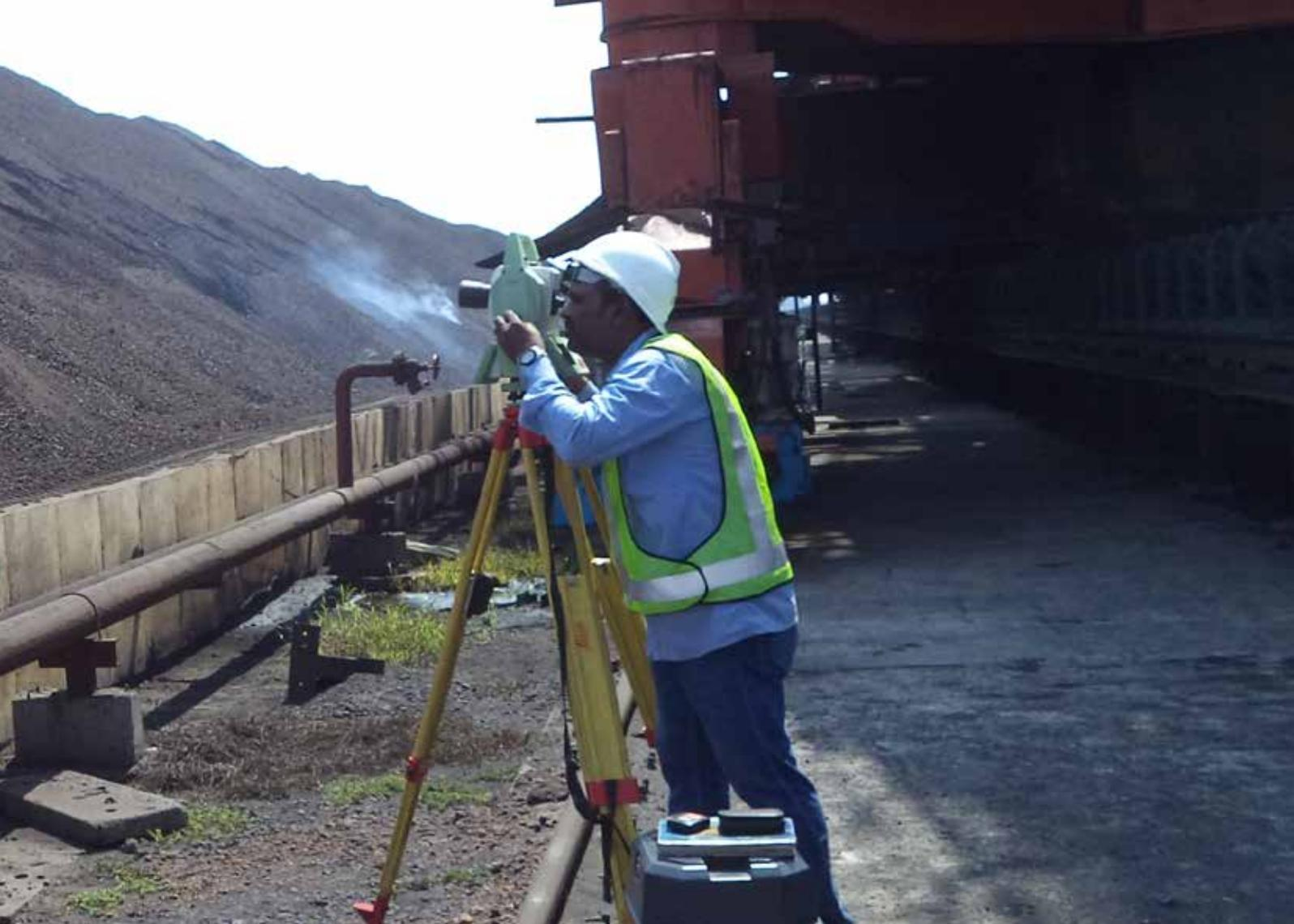
“We choose Leica MultiStation MS50 instead of a total station because we were able to achieve the accurate volume of the coal stock yard, and the report generation process is easier using Leica Infinity software. Time and cost saving was one of the main factors in this project. Optimised coal volume calculation can be achieved using the MS50,” said Nandagopal Kesavan, assistant manager of operations at TPCIL.
