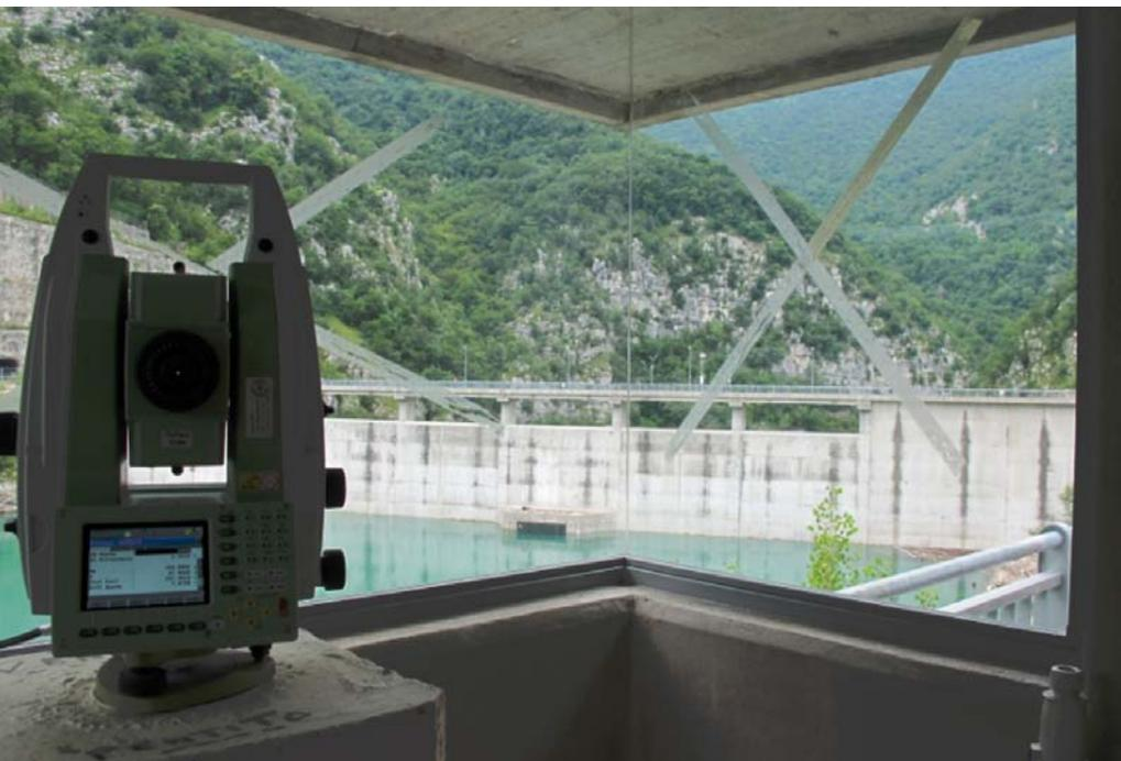
Automatic monitoring system with dual station operation with the Leica TM30 station.
