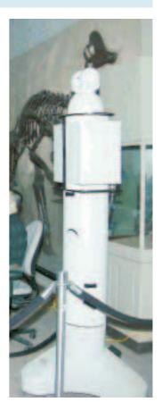
(Right): The LR200 coherent Laser radars had to be placed on towers in order to navigate around the skeleton
