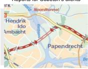
The Sophia Noordbuis Tunnel Project comprises twin-bore 4.5km (2.8 mile), 8.45m (26') diameter rail tunnels. Passing beneath the Rietbaan waterway (south-east of Rotterdam), between the towns of Zwijndrecht and Papendrecht, at approx 25m below sea level, Sophiatunnel forms a crucial link in the new strategic rail-freight line linking Europe's largest freight seaport, Europoort at Rotterdam, to the western border region of Germany.
