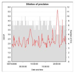
Using GPS only, the number of available satellites is between 6 and 10 with an average of approximately 7 GPS satellites being visible. The GDOP has an average of approximately 2.3 and peaks at 5.5.
