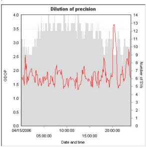
Adding GLONASS satellites increases the number of available satellites from between 8 to 14 with an average of approximately 10 or 11 satellites being visible. Similarly, the GDOP values are reduced.
