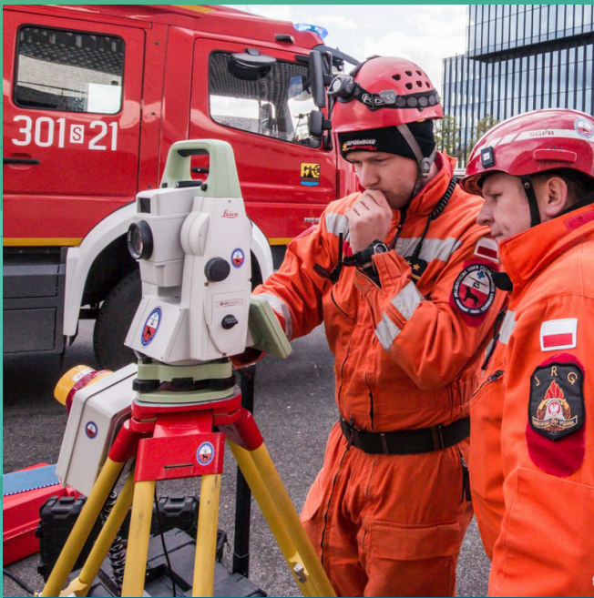
To monitor damaged structures of burned buildings that might collapse, the Polish State Fire Service uses Leica Geosystems TS16 total stations. By Paweł Krótki, Poland.
