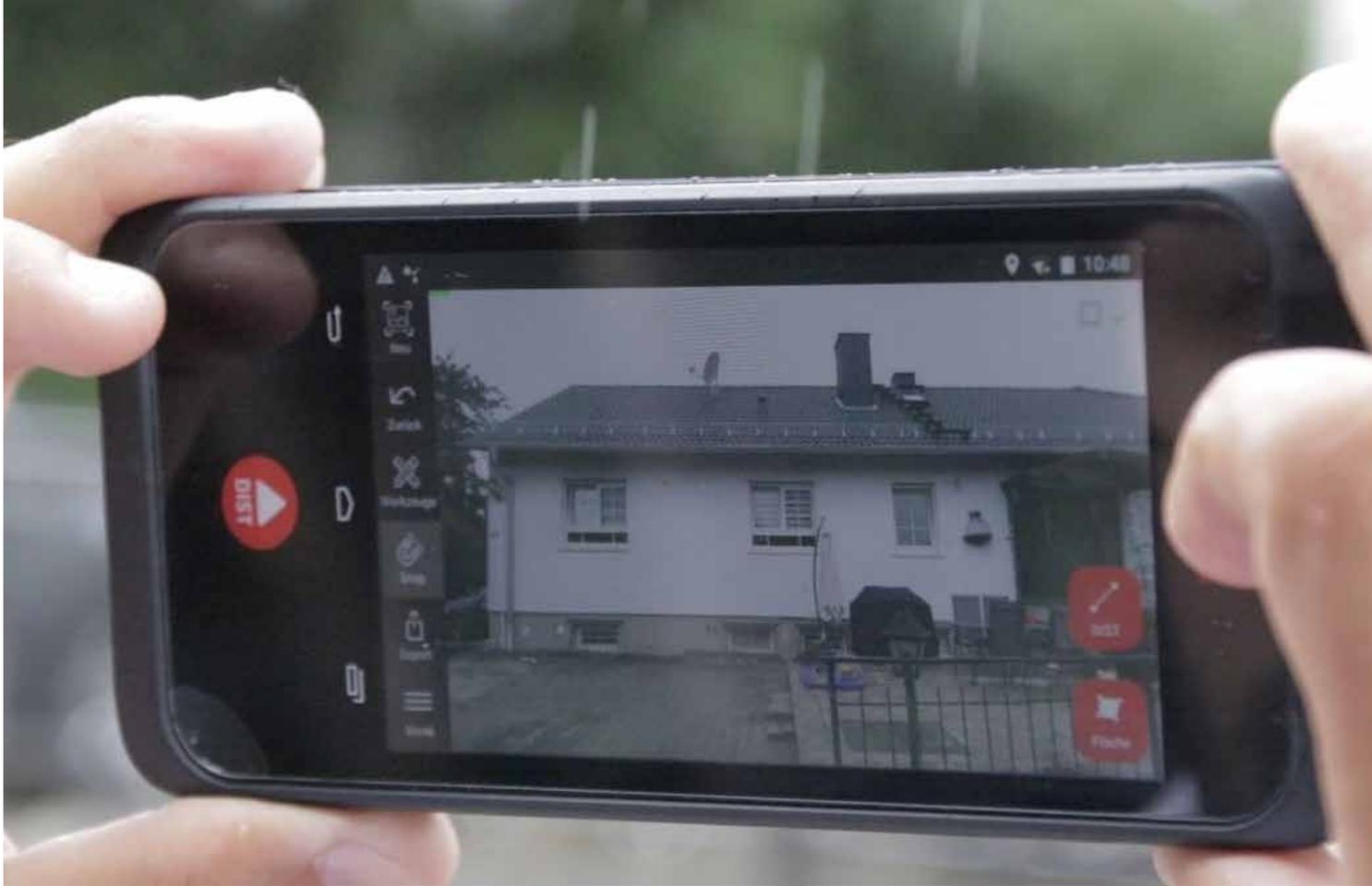
check, but variations between this and the in-picture measurements are usually less than 1 centimetre. If the process is followed correctly, meaning two images are taken, which are then overlaid, the accuracies are more than satisfactory for a scaffolder. For the final invoice, however, measurements of the actual installations are used.
