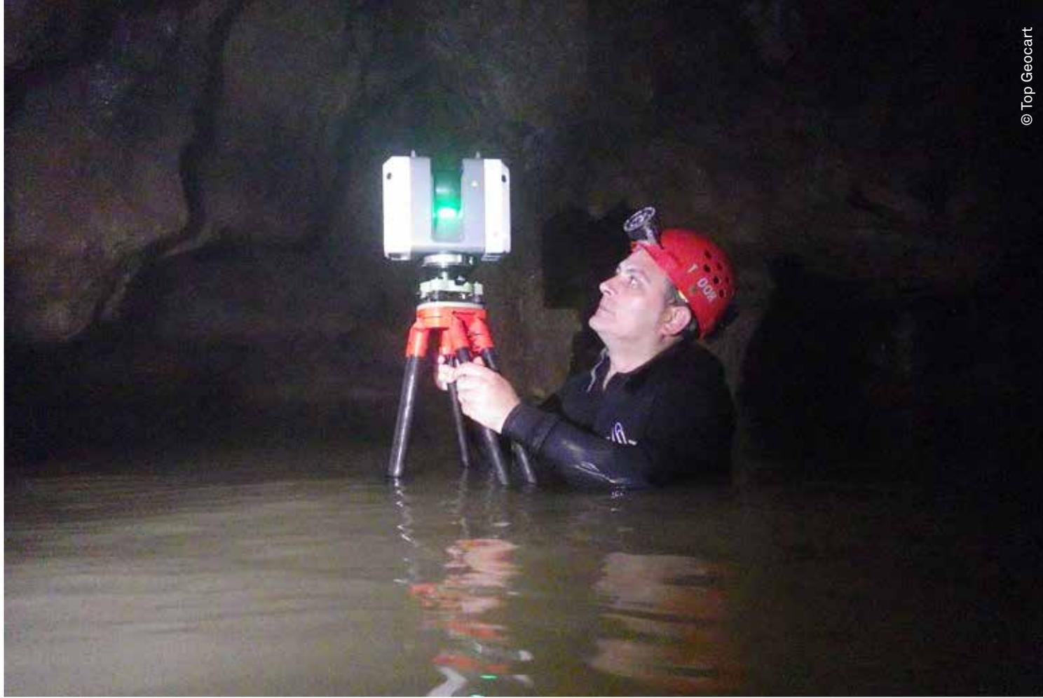
DISTO™ data, too. Together with Spelemat, Top Geocart created a unified point cloud, as Cyclone REGISTER 360 project, and exported in E57 and LGS formats to visualise it with JetStream Viewer, a light-weight point cloud viewing tool. The E57 file was imported in Leica Cyclone 3DR to create meshes and compute digital terrain models (DTM) from point clouds.
