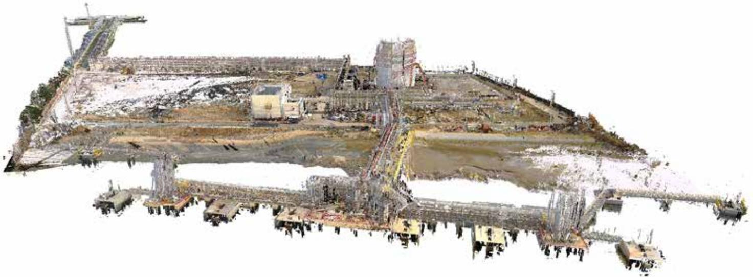
data. After collecting the point cloud data from the geodetic equipment, Portcoast used Leica Cyclone, Leica Cyclone 3DR and Leica Infinity software off-site to process the data.
